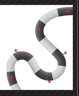
The final design is produced through rapid automated fabrication to deliver a mm-scale, ultra-soft and flexible tentacle with a patient-specific magnetic signature.
